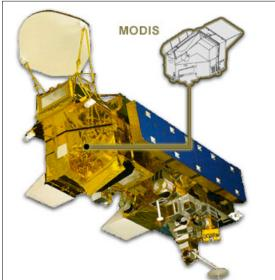
The Moderate Resolution Imaging Spectroradiometer (MODIS) instrument is designed to provide observations that scientists can use to increase understanding of global dynamics and processes occurring on the surface of the Earth and in the lower atmosphere.
