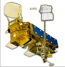
The Atmospheric Infrared Sounder (AIRS) will measure humidity, temperature, cloud properties, and greenhouse gases throughout the atmosphere. These measurements, along with others, will allow scientists and operational agencies around the world to improve weather prediction and to observe changes in Earth's climate.
