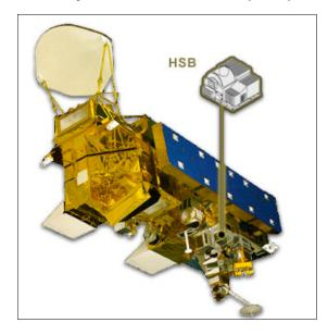
The Humidity Sounder for Brazil (HSB) will obtain humidity soundings, and measure precipitation and the total amount of water in the atmospheric column beneath the satellite. HSB is particularly important because of its capability to obtain humidity profiles under conditions of heavy cloud cover. HSB has four channels, and the data from the instrument will have horizontal resolutions of 13.5 km (8.3 miles).
