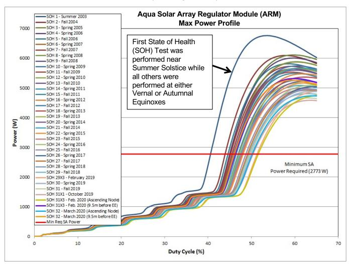
When comparing State Of Health (SOH) tests performed Near Equinoxes, Solar Array degradation has been as expected given the age of the spacecraft.
