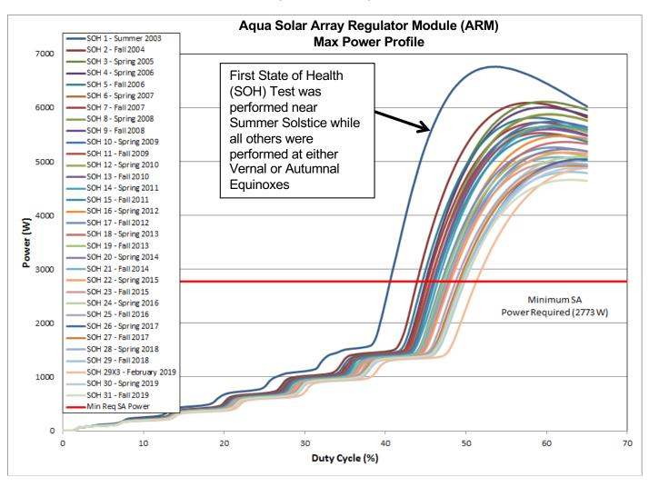
When comparing State Of Health (SOH) tests performed Near Equinoxes, Solar Array degradation has been minimal. The Solar Array can provide sufficient power at least until 2025, even with an anticipated exit from the A-Train in 2022.
