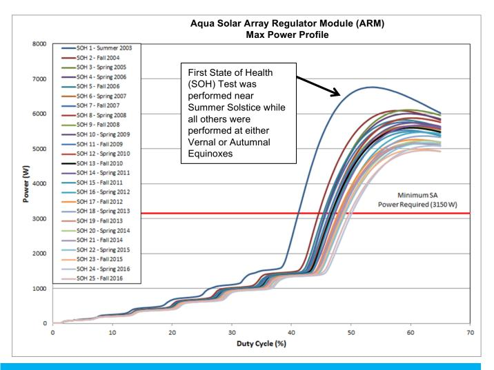
When comparing State Of Health (SOH) tests performed Near Equinoxes, Solar Array degradation has been minimal. Solar Array can provide sufficient power through 2028.
